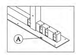
Slide cross beam over both tabs on leg.
